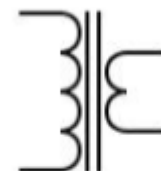
Gambar 3. Skema transformator step-down
