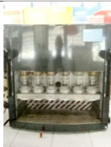
Fat level analysis using soxtech
