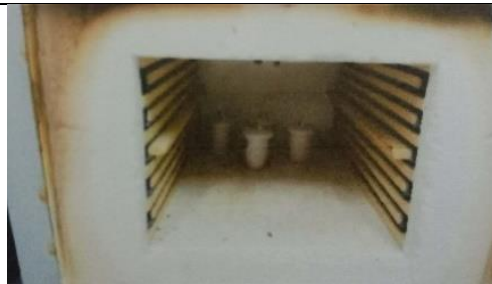
Removed a cup of porcelain ash and cooled in a decicator for 30 minutes
