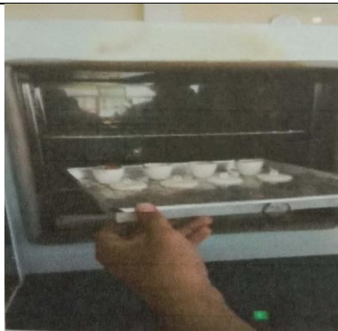
Put in the oven at a temperature of 100°C for 24 hours
