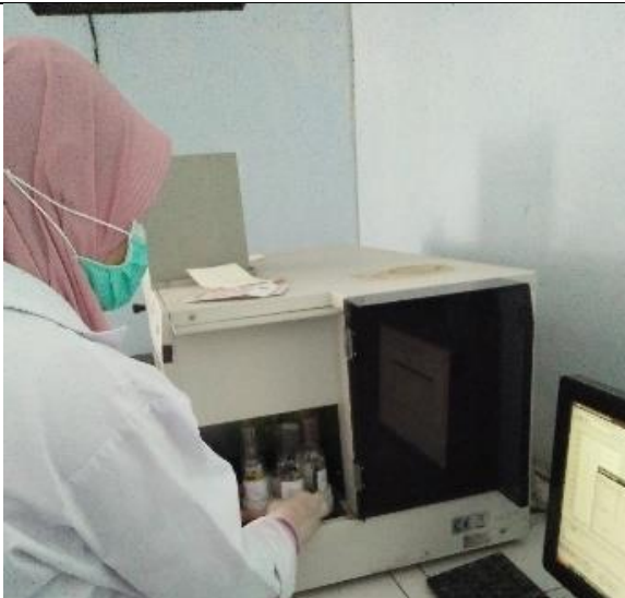
Hollow cathode lamp replacement on AAS
